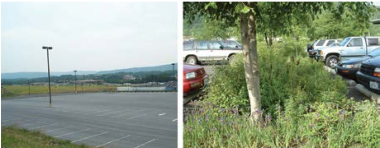
Figure 40. The harsh environment of a parking lot (left) can be tempered by including an interior planting strip that allows trees to share rooting space (right).
